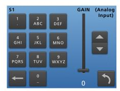
Gain is used to match the analog input levels to the Digital sources. Some Analog sources have large variation in output levels. The OdB default setting is suitable for connection to high output devices like CD players, while the standard level (1Vrms) is achieved by setting the gain to +6dB. The Gain slider (and source button) will flash red if the gain is set to high and distortion is detected. Select the Back arrow to return to the System Settings Page.
