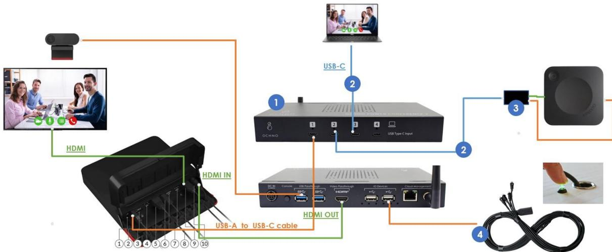
In this setup, both the CX wireless connection and the wired USB-C connection can be used to both run a MTR-hosted meeting or run a meeting from the laptop (BYOD).
