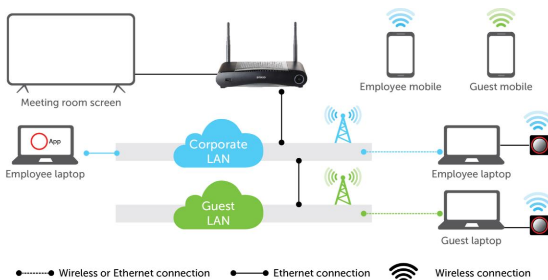
Figure: Enterprise network integration topology diagram, for this example the corporate LAN is used
